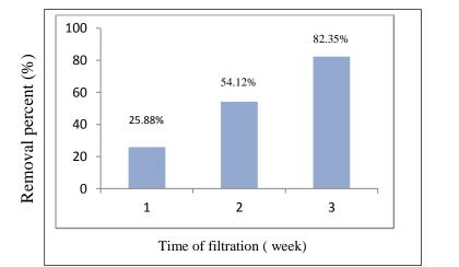
Figure 7: The plot of percent removal of lead vs time of filtration by using activated rice husk charcoal (Site -2)
